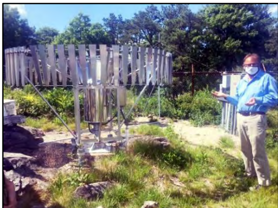
Equipment to measure rainwater. The metal hanging on the side keeps the rain from blowing, directing it straight into the measuring tube. Photo by Ellen Thompson
