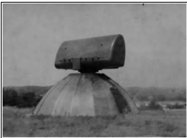
Acquisition radar. This would bounce electronic signals off airplanes to determine "friend or foe." Friendly aircraft would respond with a specific signal that functioned as a secret handshake. (Burlington installation) 2
