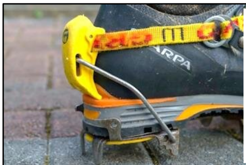
Technical crampons use a large clip (shown in yellow) that fits into a groove on the heel of the boot.
