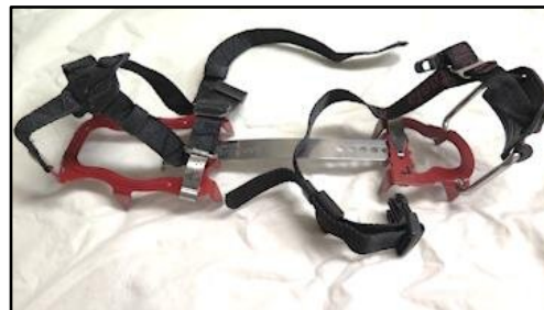
The toe and heel metal frames are connected by an adjustable bar.
